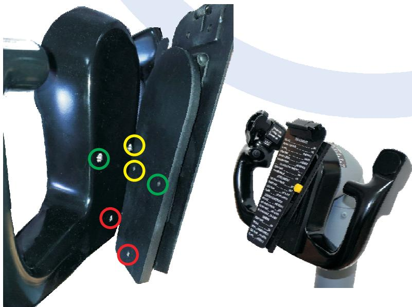
2. Extract the front cover of your yoke (V2) with a flat screw driver untightening the 3 M4 black screws from the back of the yoke
