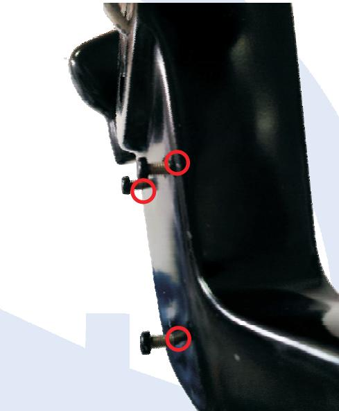
4. If your yoke is V1 or is not Opencockpits made, you should extract the cover (step 2), do a stencil with the maps holder and drill the yoke with a lot of care and go to step 3.
